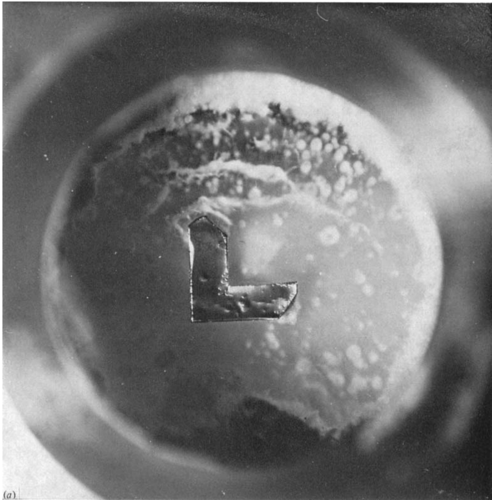
FIGURE 24. Liquefaction front with various conditions. (a) PP3, T_0 = 130^\circ\text{C} , P_0 = 0.99 bar, M_I = 2.05 , equilibrium moisture y_1 = 15\% . Lighting arrangement B , left-hand light only. Frame diameter 50 mm. (b) PP3, T_0 = 80^\circ\text{C} , P_0 = 0.24 bar, M_I = 2.70 , y_1 = 16\% . Lighting arrangement B . Frame diameter 70 mm. (c) FC-40, T_0 = 150^\circ\text{C} , P_0 = 0.33 bar, M_I = 2.50 , y_1 = 27\% . Arrangement B . Frame diameter 70 mm.
